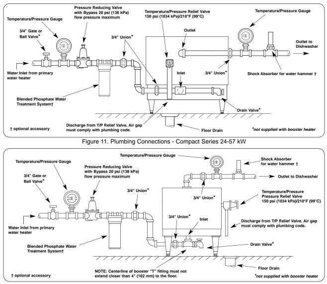
Figure 12. Plumbing Connections - Mini-Compact Models
