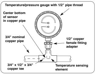
Figure 15. Alternate Temperature/Pressure Gauge Installation
