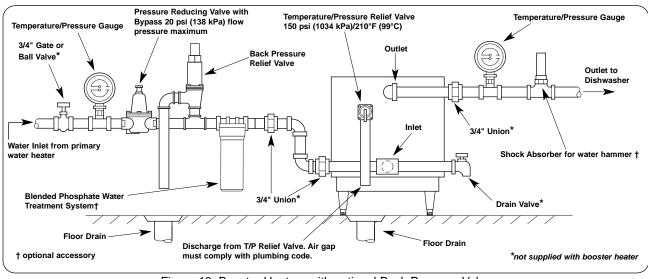
Figure 13. Booster Heaters with optional Back Pressure Valve
