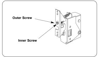
Figure 19. Thermostat Adjustment
