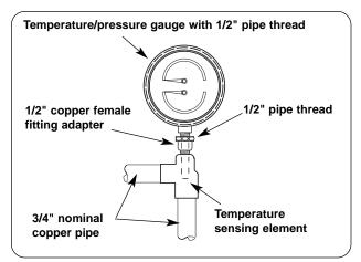
Figure 14. Recommended Temperature/Pressure Gauge Installation
