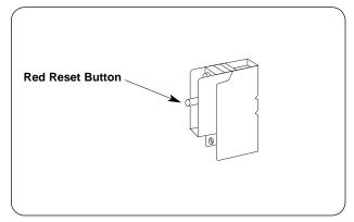
Figure 20. High Temperature Limit Safety Switch
