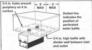
Figure 5. FR With Water Baffle
