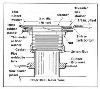
Figure 8. Installation Sink Strainer
