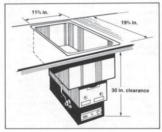
Figure 7. Therma-Corn Model FRC-I
