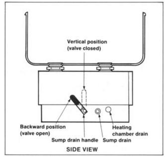
Figure 9. Heater Drain Controls
