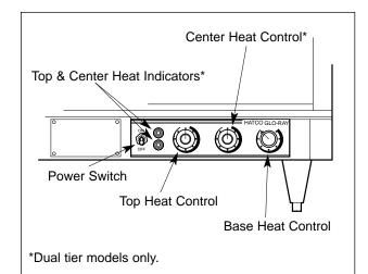
Figure 11. Control Panel – Non-Humidified Models
