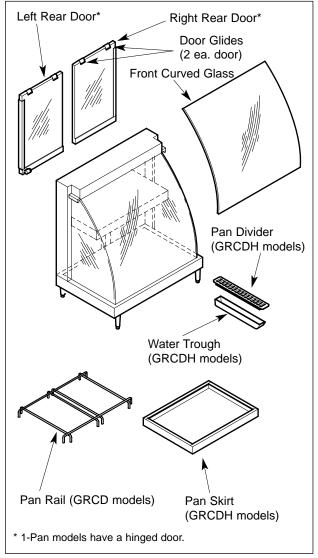
Figure 9. Exploded View - GRCD Models
