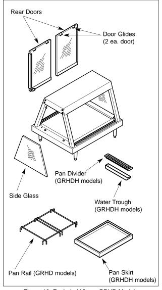
Figure 10. Exploded View - GRHD Models
