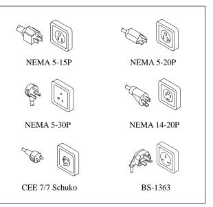
Figure 5. Plug Configurations
