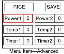
b. Turn the Control knob until the desired value appears for the cooking control method. Push the Control Knob to save the value.
