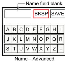
8. Turn the Control Knob until SAVE is highlighted in red, then push the Control Knob to save the menu item name.
