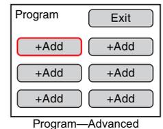
5. Turn the Control Knob clockwise until +ADD is highlighted in red, then push the Control Knob to name the menu item.
