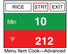
5. To stop cooking during a menu item sequence, turn the Control Knob to highlight EXIT in red, then push the Control Knob to stop the sequence.
