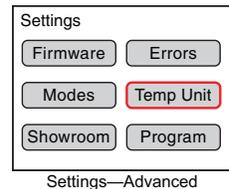
3. Turn the Control Knob clockwise until TEMP UNIT is highlighted in red, then push the Control Knob to select TEMP UNIT.
