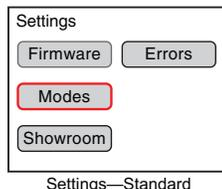
3. Turn the Control Knob clockwise until MODES is highlighted in red, then push the Control Knob to select MODES.
