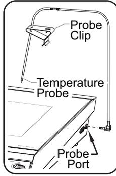
2. Insert/submerge the bottom 1" (25 mm) of the probe into the food being cooked.
