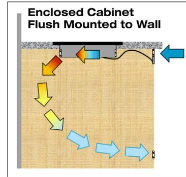
Cabinets should be sufficiently open to allow fresh air to cool the units. Two areas equal to 20 sq. inches (129 sq. cm) each should be provided for each unit. These should be located as close as possible to the intake
